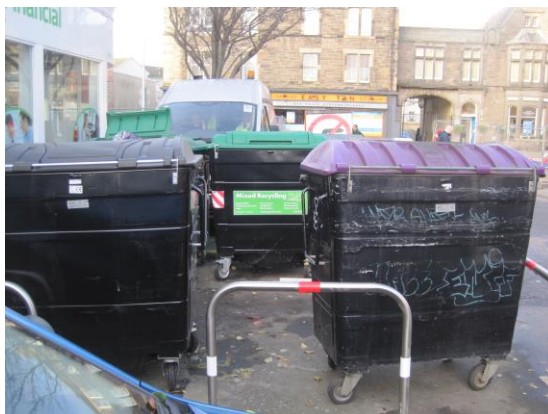
Figure 8 Example bin hub as built outside the study area in Smith Place. This is an “in nose” (end on) parking layout’ configuration. A larger gap can be seen between bins than shown on concept design.
